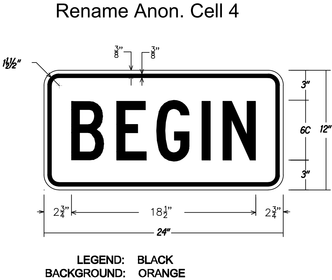
TYPICAL DETAIL FOR CONSTRUCTION SIGNS ON TWO LANE OR MULTILANE UNDIVIDED HIGH SPEED HIGHWAY
